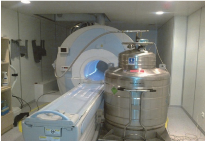
Photo 6. The process of replenishing helium levels in an MRI machine
