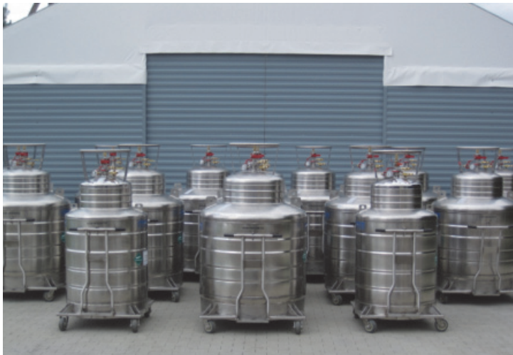
Photo 3. A set of cryogenic tanks for the transport of liquid helium
